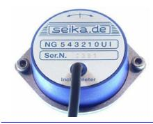
Inclinometers of high measuring accuracy for inclination measurement in the ranges of  $\pm 10$ ,  $\pm 30$  and  $\pm 80$  degrees with a non-amplified, non-conditioned output signal
