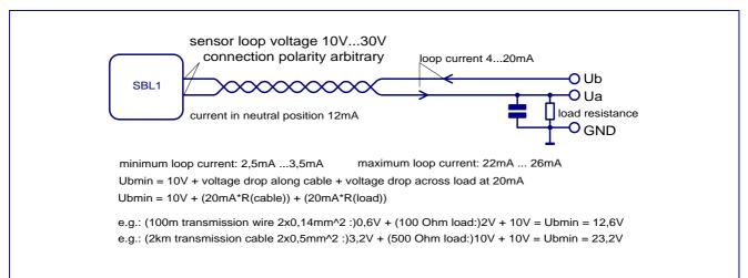
Since the supply voltage of the SBL1 feeds off the loop current (the SBL1 requires 3mA at the most), a voltage of 9V across the SBL1 terminals must be guaranteed to ensure correct functionality even for the maximum loop current of 24mA (maximum voltage drop across transmission line and load resistor).
