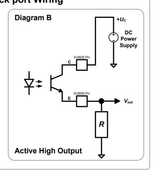
In the Diagram B Active High Output, the output signal  $V_{\rm out}$  switches to  $+U_{\rm C}$  when the corresponding LED is ON. When the output signal  $V_{\rm out}$  is switched to GND, its value is lower than 0.2 V. When the output signal  $V_{\rm out}$  is switched to  $+U_{\rm C}$ , its value is equal to  $+U_{\rm C}$ .
